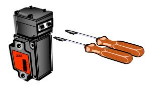
Fig. 1: Attempted actuation using two identical objects
