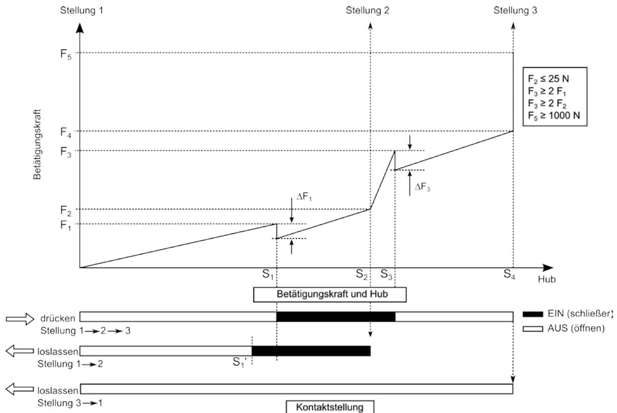
Figure 1: Representation of the operating characteristics of a three-position enabling switch/ device configured with a foot switch.
